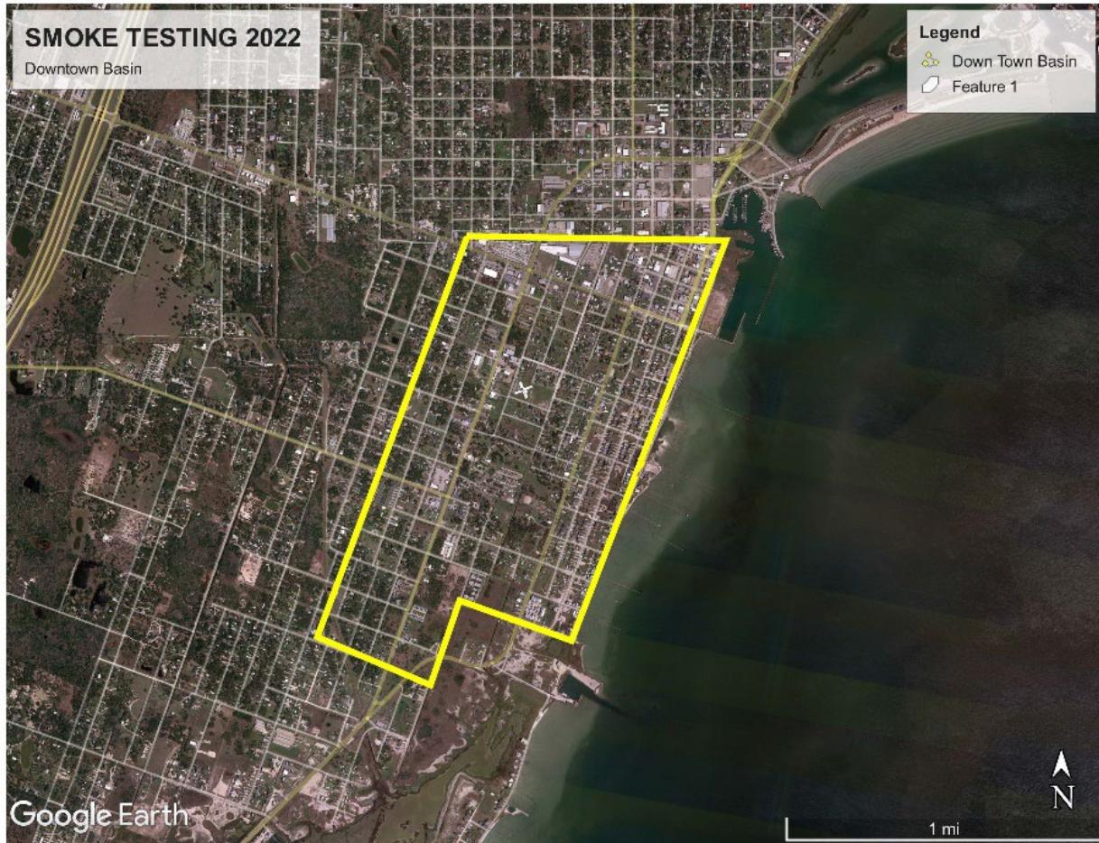
Each year sewer basins are tested to ensure that only sewer flows enter these lines. Large rainfall events force rainwater into the sewer system and it is costly to treat. Smoke testing identifies those areas where infiltration is occurring and improves our system by indicating where repairs are to be made.
