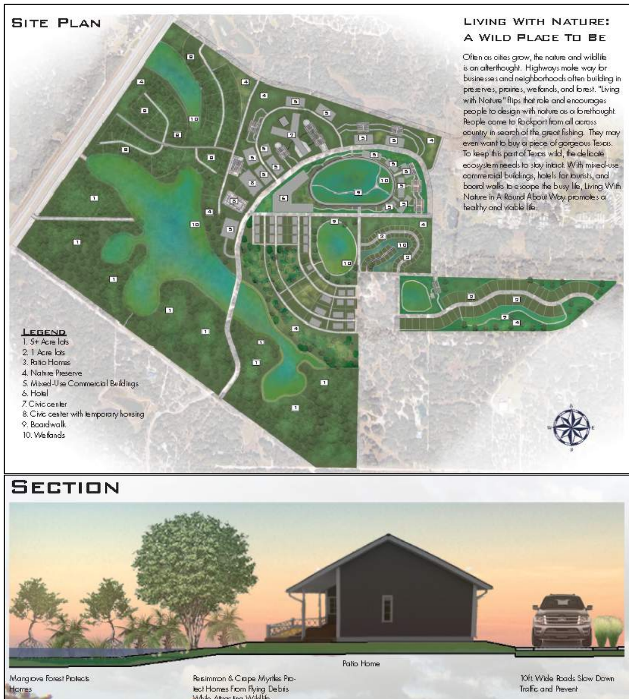
Figure 30: T-4 Transect zone example mixed-use project combining development with nature. The design features commercial, hotel, and residential development surrounding by a boardwalk system, mangroves, and wetlands. Source: Ryan Beatty.
