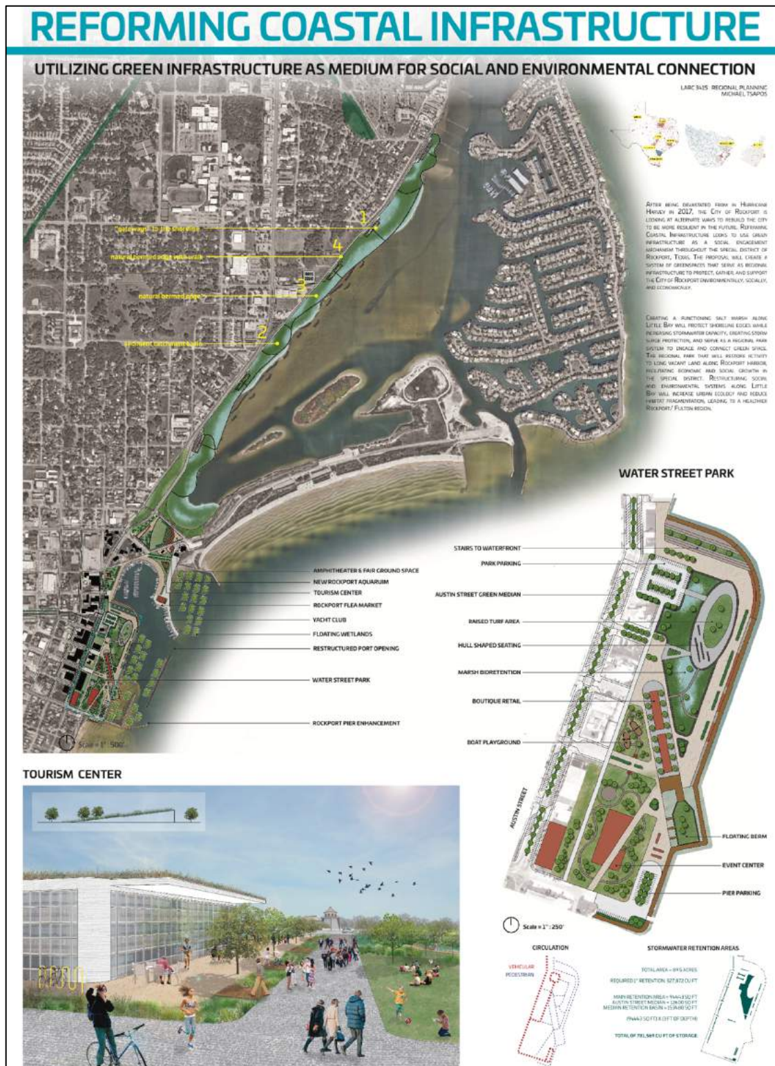
Figure 38: SD-Special District Transect zone example project featuring a created salt marsh along Little Bay to increase stormwater capacity, protect from storm surge, and serve as a regional park system. A berm system, sediment traps, and floating wetlands protect the existing retail areas and proposed aquarium, amphitheater, yacht club, and park. Source: Michael Tsapos.
